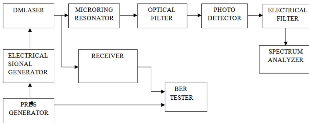
**Fig.3.1.**Block schematic of photonic system for THz signal generation using DM laser
