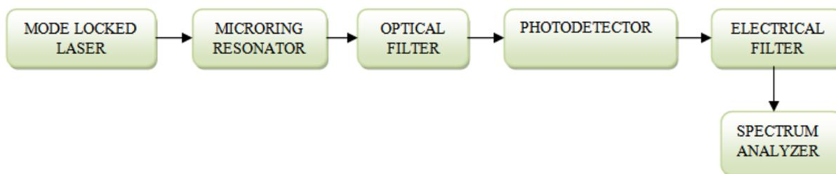
**Fig 2.1** Block schematic of photonic system for THz signal generation using MLL
